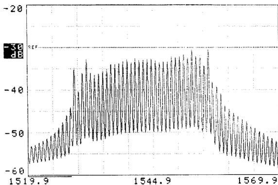
Fig. 6 Output with oscillation employing both SOA gain axes.
