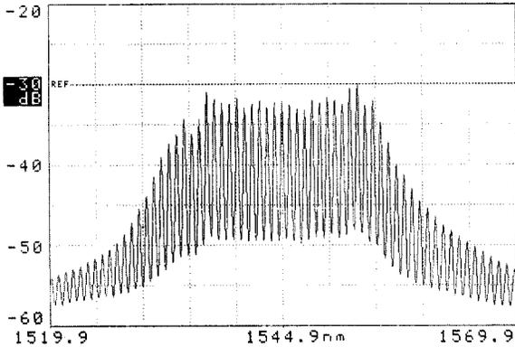
Fig. 3 Optical spectrum of the multi-wavelength laser.
