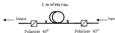
Fig. 1 The PM fiber, comb filter.
