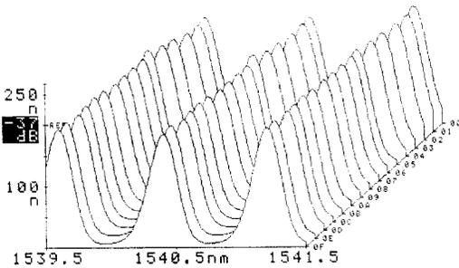
Fig. 5 Output time evolution over 90 min.
