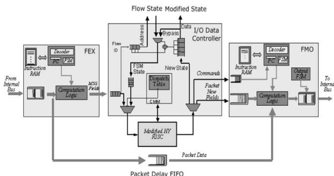
Fig. 1. Programmable processing functional model and block diagram.
