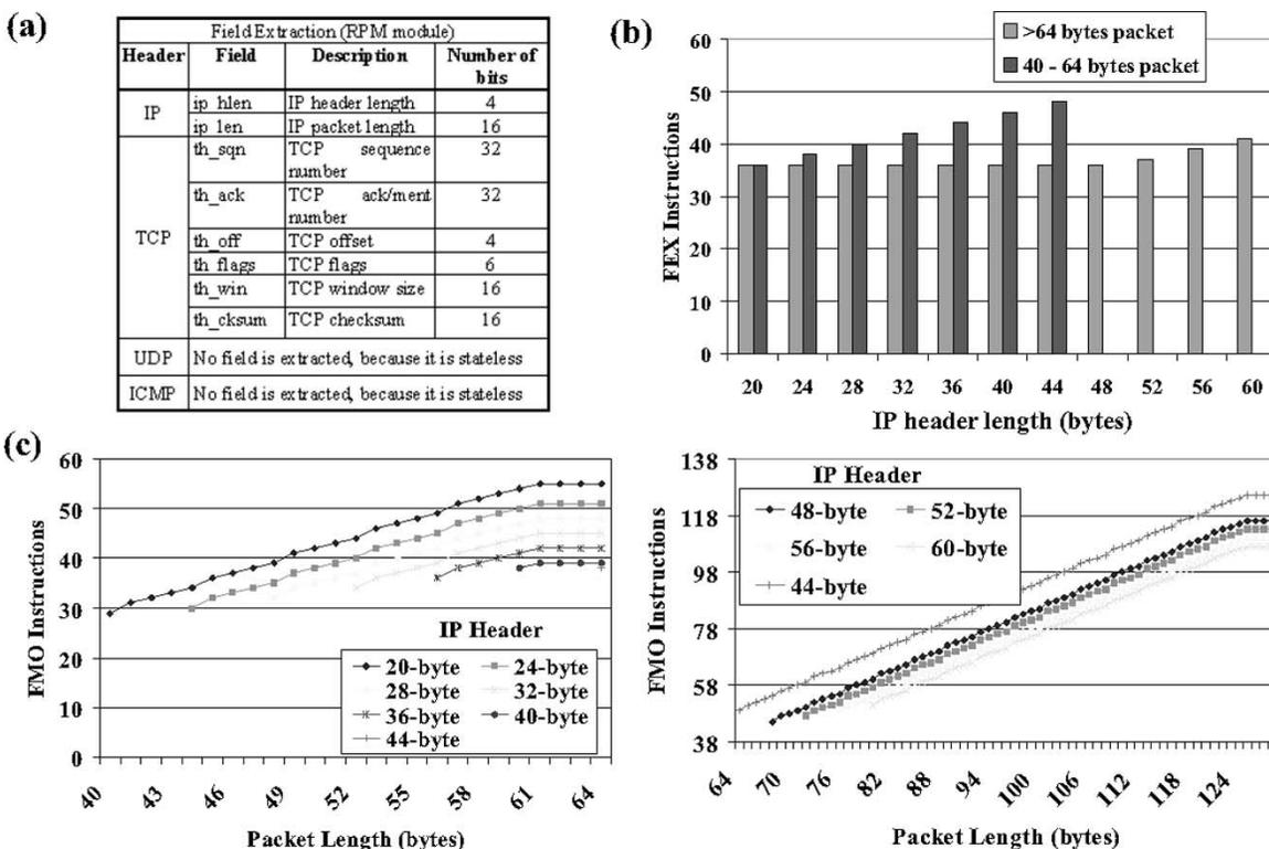
Fig. 2. Fields extracted by FEX and number of instructions and processing time for the FEX/FMO.
