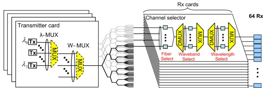
Fig. 1 Implementation of an optimal  $64 \times 64$  optical interconnect with discretely-tunable receivers.
