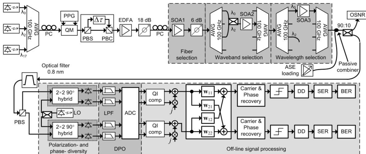
Fig. 3 Experimental setup and DSP algorithms.
