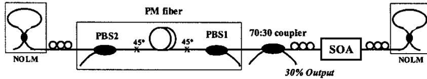
Figure 2: Experimental layout of multi-wavelength linear cavity laser.
