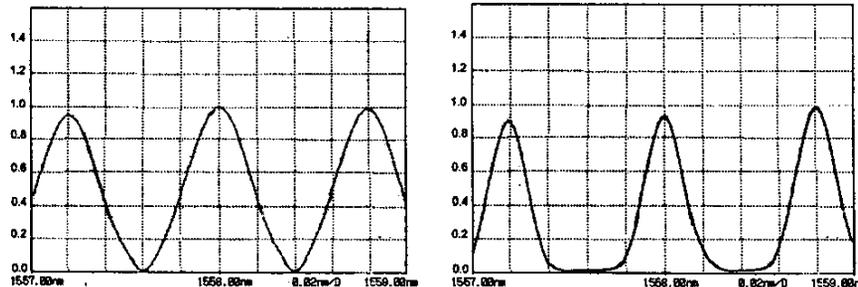
Figure 4: (a) and (b): Single and double pass transmission through the Polarization Maintaining Fibre Lyot Filter.
