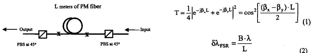
Figure 1: (a) The PM fiber Lyot filter and (b) Transmission function (1) and free spectral range of the filter (2)
