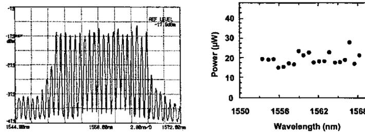
Figure 3: (a) Output optical spectrum of the multi-wavelength (b) Optical power variation versus wavelength.
