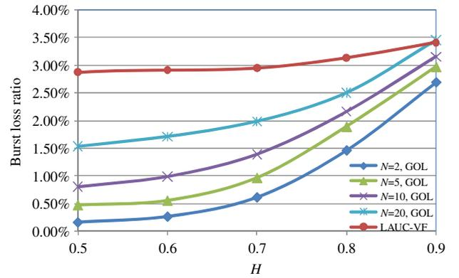
Fig. 8. (Color online) Burst loss ratio versus Hurst parameter for predictive reservation and JET. We kept the load constant, at 0.7.
