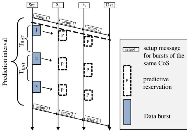
Fig. 2. (Color online) Timing considerations of the proposed predictive reservation protocol. Dots denote burst reservations based on predictions, which are communicated to all nodes across the path with a single **setup** message. Actual bursts arrive at a later (predicted) time.
