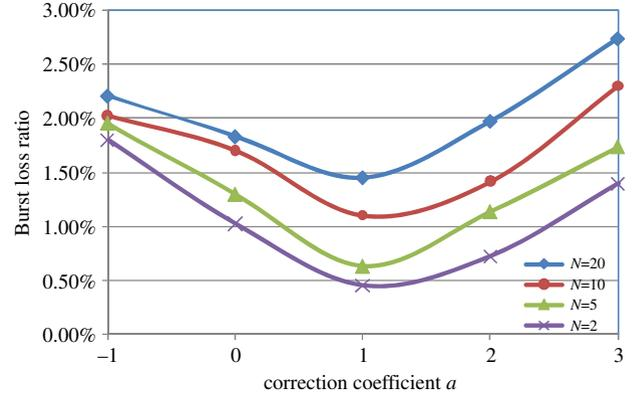
Fig. 6. (Color online) Burst loss ratio for different  $\alpha$  coefficient of the correction parameter  $\delta$ , for a constant 0.7 load and 0.7 Hurst parameter.
