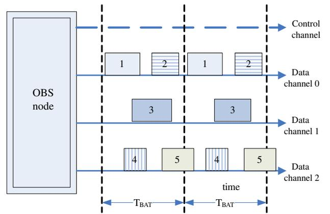
Fig. 1. (Color online) Link scheduler utilization profile, repeated periodically on a  $T_{BAT}$  basis.
