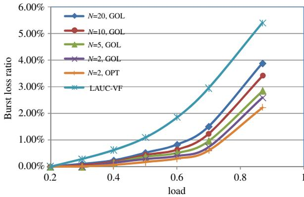
Fig. 7. (Color online) Burst loss ratio versus load comparison of proposed reservation protocol and JET, with different sampling periods  $N$  and scheduling algorithms. The Hurst parameter was kept constant at  $H = 0.7$ .
