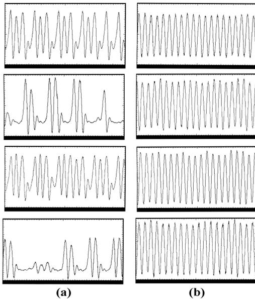
By electrically delaying the initial pulse trains from the DFB's by 33.3 ps, it was also possible to recover clock at 30 GHz. In this instance the pulse width of the recovered pulse train was 12 ps. Further improvements in the output pulses may be obtained by using the design guidelines for optimizing the cavity length and dispersion discussed in ref. /10/. The clock recovery circuit discussed so far is a tuned
