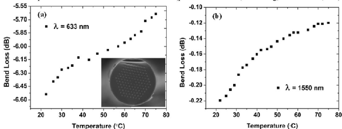
Fig. 1 Power recovery of the hybrid PCF under a constant bend diameter of 4.8 cm at (a)  $633 \text{ nm}$  and (b)  $1550 \text{ nm}$  wavelength. Inset: SEM image of the PDMS-filled PCF.
